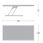
Table with upholstered desktop in black LEATHER. Desktop frame made in solid oak. Polished stainless steel 60° inclined Ø 250mm column base attached to top and bottom plates of 15 mm thickness aluminium. Bottom support plated in matt stainless steel. Base provided with adjustable feet levelers.
