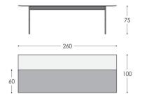
25 mm rectangular table top and partial overtop. Top resting on two sides joined together by an upper metal structure. Sides include an internal metal structure, visible at the edges.
